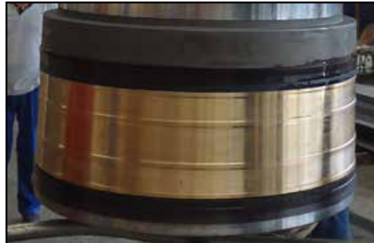
Bearing grooves being machined in the old bushing.
